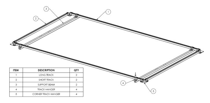
Use as many people as needed to flip and lift frame assembly. Adjust positions of support beams as needed and set support beams on top of vertical mounting bracket that you previously installed.
